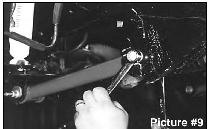
and replace the lower links with new Rugged Ridge extended links (one side at a time). See picture #9. Only start these bolts and nuts, do not tighten at this time. NOTE: so that the links may be greased while on the vehicle, install them with the zirc fittings positioned as follows: **front** eye of link has fitting pointing out the **end**, **rear** eye of link should have the fitting pointing **down**.
