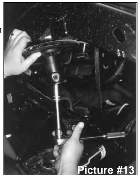
3. After removing both coil springs, remove the bump stops (it may help to use channel lock pliers working bump stop back and forth). Remove 10mm bolt from inside bump stop cup. Install bump stop spacer and original cup using furnished 10mm bolts. Reinstall factory bump stop. (See picture #13.)
