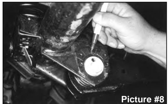
10. Install drive-in zirc fittings in each end of links by using a 1/4" socket over the fitting, tap with a hammer until fitting is completely tapped in.
