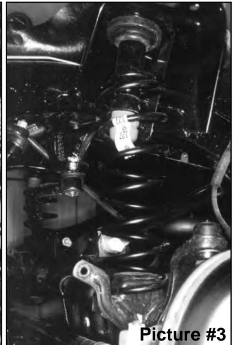
4. Now remove both coil springs. Remove upper bump stop (use channel lock pliers working bump stop back and forth).
