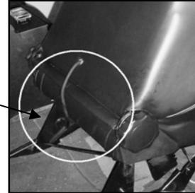
Step(10) Velcro straps have been supplied on the left and right side of the seat so that the air pump can be mounted in relation to what side of the vehicle the seat has been mounted. For the drivers side it is recommended that it be placed on the right side of the seat (inboard). When attached to the passenger side it is suggested to use the left side of the seat. By locating the air pump to these spots you will not hit them when entering or exiting of the vehicle.
